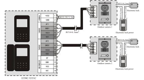
Connection diagram between indoor monitor and outdoor camera (1pc indoor monitor + 2pcs outdoor camera + 1pc extension unit)
