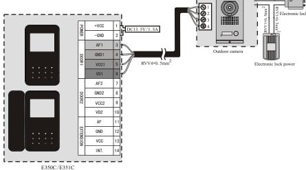
Connection diagram between indoor monitor and outdoor camera (1pc indoor monitor + 2pcs outdoor camera)
